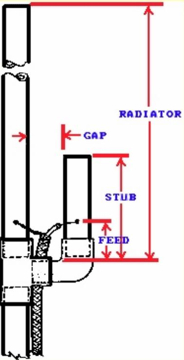
The diagram illustrates the physical structure of a J-Pole antenna. It consists of a vertical radiator tube, a horizontal gap, a driven stud, and a feedpoint. Red arrows indicate the lengths of the radiator, gap, and stub. Blue arrows indicate the feedpoint. The diagram is labeled with 'RADIATOR', 'GAP', 'STUB', and 'FEED'.
